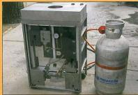
For the FURANFLEX® technology only special tools and steam generators can be used, supplied by Kompozitor
