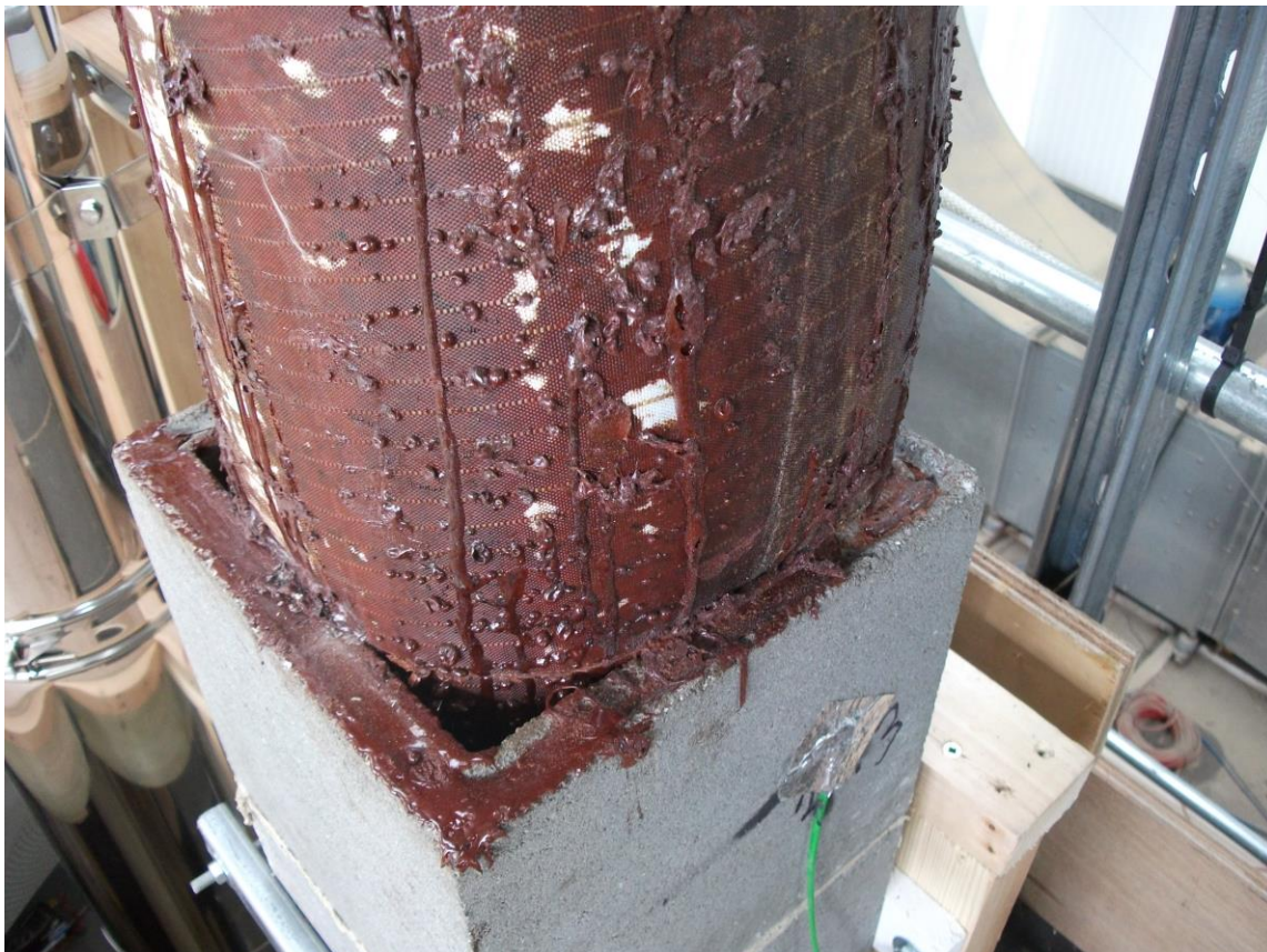
Photograph 3 (Top section after installation of liner, to be cut off level with test chimney)
