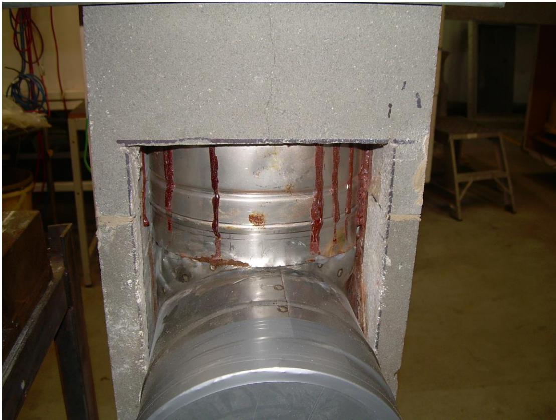
Photograph 2 (Tee connection for gas tightness test)
